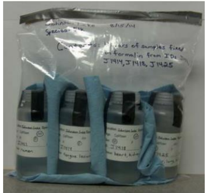
Figure 2. Absorbent material placed between the primary sample containers and the secondary bag.
